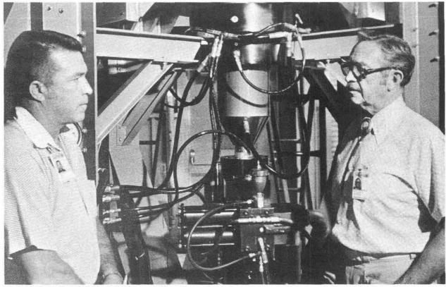
THE LOW FREQUENCY SHOCK and vibration encountered during transportation and handling can be simulated (with a displacement up to eight inches) on this vertical shaker in Area III. Operator Lynn Loveland (1546) and Bill Gardner, Director of Development Testing 1500, discuss upcoming tests on containers being developed for rail and truck shipment of nuclear materials.
